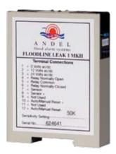
The Floodline Leak 1.MkII is a self-contained single zone leak detection module specially designed for incorporation into other control/ alarm systems, air conditioning units and BMS etc. The module can be used with all Floodline sensors.
