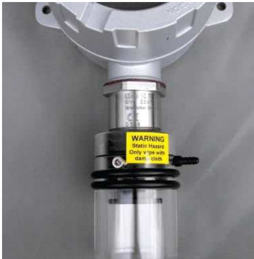
ATEX/IECEX Detector fitted with an IGD splash guard
