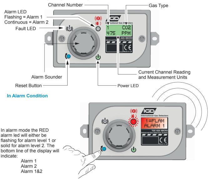
The back light will flash red and the display will indicate which alarm level and which channel is in alarm. The sounder will also activate. Pressing the button will silence the sounder and mute the relay nodes if connected as indicated in table 1. If the gas is still breaching the alarm threshold it will not be possible to reset the alarm
