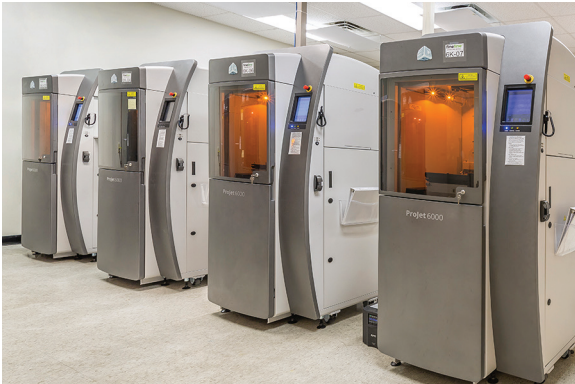
High-speed stereolithography equipment can rapidly produce parts with excellent surface finishes that mimic plastics like ABS, polycarbonate and polypropylene.
