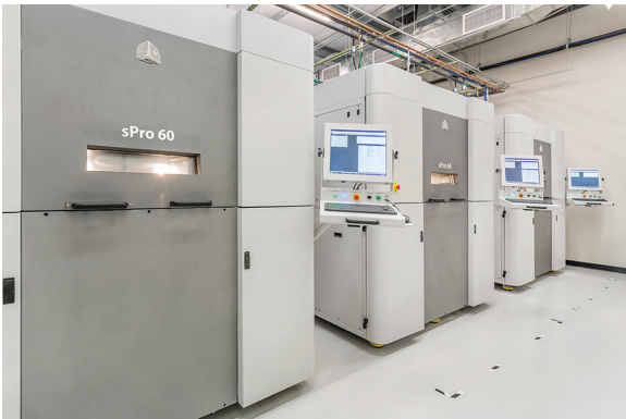
Selective laser sintering fuses layers of fine powder to form parts in various grades of nylon thermoplastics.
