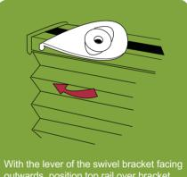
outwards, position top rail over bracket which should then be rotated to lock the rail in place.
