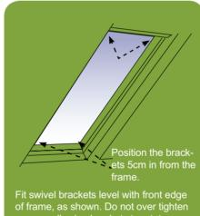
Fit swivel brackets level with front edge of frame, as shown. Do not over tighten screws, allowing brackets to rotate
