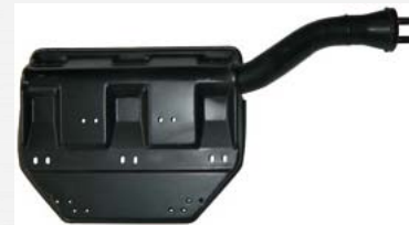
SCA070 WING STAY - RH *BOLTS POSITIONED AT 6 & 12 4x2 REAR 6x2 FRONT 6x2 MIDDLE
