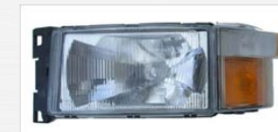
SCA090 HEADLIGHT - LH *WITH INDICATOR & WIRING LOOM
