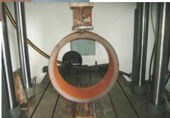
Opposite: Pipe being type tested in accordance with EN295-7 Clause 4.8 Strength
