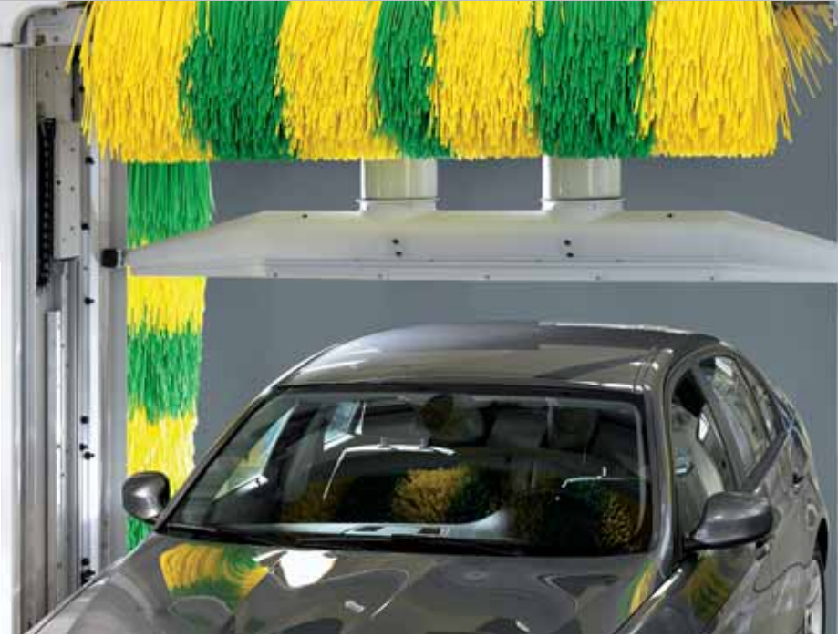
Roof blower Contour-following without additional light barriers. Optimal drying distance ensured via memory data transfer.
