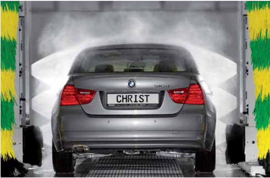
Side high-pressure 85 bar Vehicle sides are cleaned, soaked and freed of coarse dirt particles before the main wash with three high-pressure jets on each side of the unit, laying the foundation for a gentle wash.
