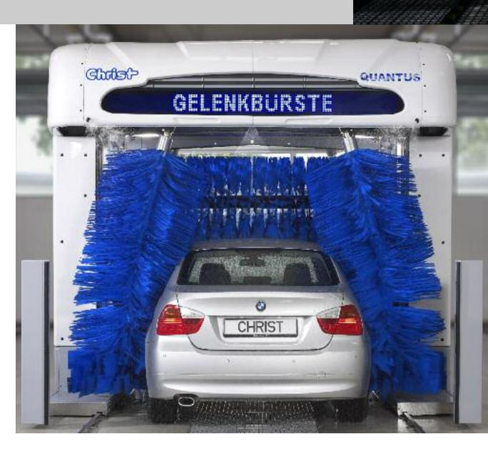
The tried and true jointed brush device only available at Christ AG awards vehicles with the best wash results during the forward and return cycle. Evenly applied pressure and optimum identification of the vehicle's contours guarantee gentle cleaning.
