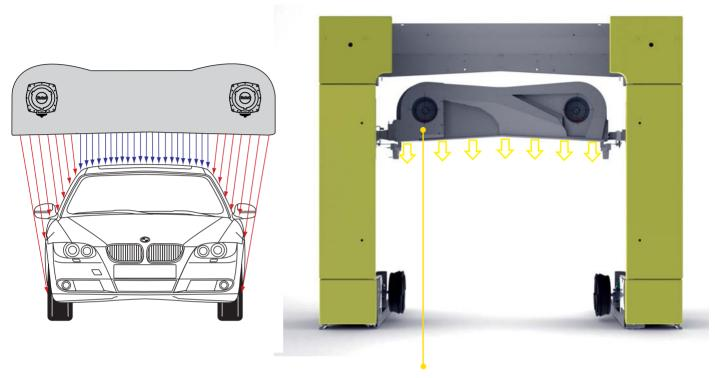
The roof jet of the novel DIVO blower is also able to dry the vehicle's side surfaces.
