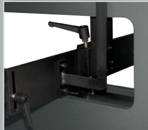
Limit stop system in Y direction Mobile, 2 guide shafts in press body.
