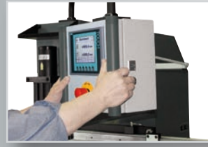
Pivoting control panel with two-hand operation
