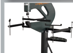
Pivoting support arms, height adjustable, each with 3 rubber supports (option)
