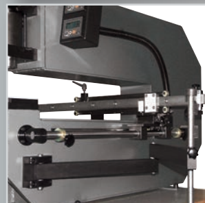
Length and depth limit stops guided in double ball bearing slides on both sides. 2 adjustable limit stops right and left on the Y-axis.
