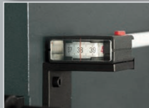
Tape measure display for Y-axis
