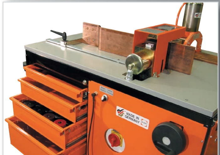
4 tool draws with compartments for punches and dies are fitted to the trolley.
