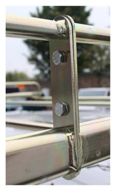
Bolt the front sections of side rails to the rears using the M6 fixings supplied and again shuffle the front brackets about if necessary before finally tightening the entire rack.
