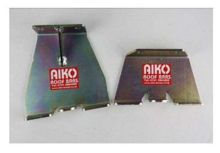
The brackets are shown here as if you are looking at the left hand/near side of your vehicle. Please note that the front brackets are taller, and are shaped to follow the slope of your roof. (This arrangement keeps your bars parallel to the road surface so that when you put large sheets of material up there, your van will neither try to take off nor drive you into the road- both of which are known in engineering terms as 'bad'.)
