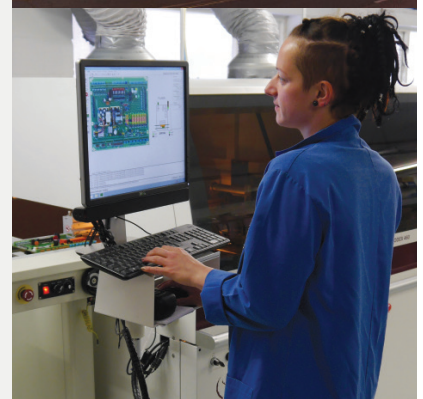
Selective soldering greatly increases repeatability
