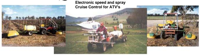
QuadCruise is an electronic cruise control that enables you to accurately control the speed of your ATV from as low as 3mph (4km/h) right up to 15mph (25km/h) and it can even provide power manually or automatically to your ancilliary equipment.
