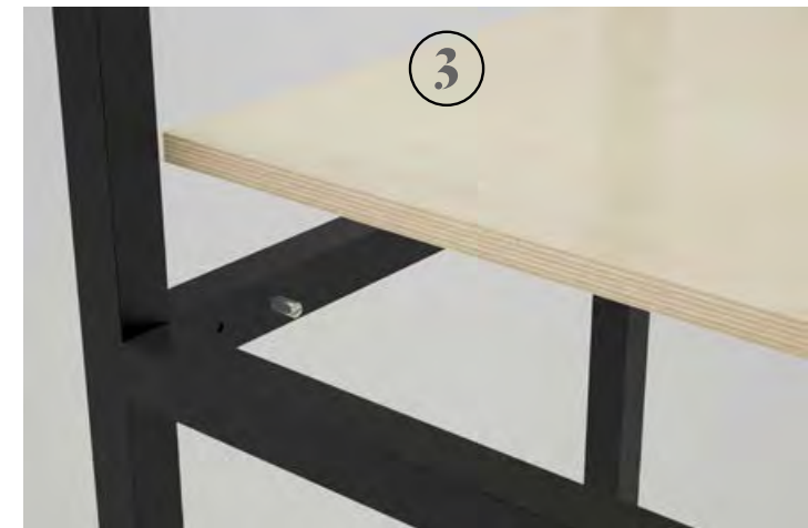
The shelf sits on top of the shelf pegs. Areas of the underside of the shelf are routed to ensure the top of the shelf sits flush with the top edge of the 25mm profile.
