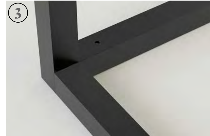
The third profile slides over the connector, making sure it's aligned with the grub screw hole. By tightening the grub screw through a pre-drilled hole, the connector expands to lock the profile in place.
