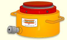
cylinder. The second type is 'pot design' used when the overall height of the unit needs to be reduced to a minimum, the disadvantage is that the cylinder is more vulnerable to damage, the piston has no end-stop and the lateral restraint capacity is greatly reduced. Both types are normally fitted with spherical swivel heads to ensure that the load is transmitted centrally through the hydraulic jacks ram regardless of any slight misalignment between the top and bottom bearing surfaces.
