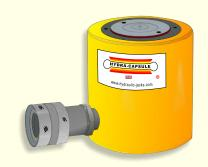
to increase its horizontal grip, we recommend that customers use a thin plywood packer between the ram and load contact area. The jack should only be operated between parallel surfaces, if this isn't the case then use of a taper shim which must cover the full ram area or install and level a steel plate bedded on a high strength mortar or grout.
