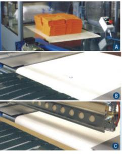
Collation of four stacks of table napkins, automatically in-fed (A)
