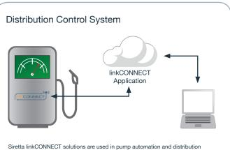
Siretta intkCONNECT solutions are used in pump automation and distribution control system projects where authorisation to distribute fuel / oil / electricity is required via credit card payment or validated company credit account. The linkCONNECT solution provides a point to point link to the distribution point and provides a real time device status which can be used to authorise payments and initiate delivery of the service.
