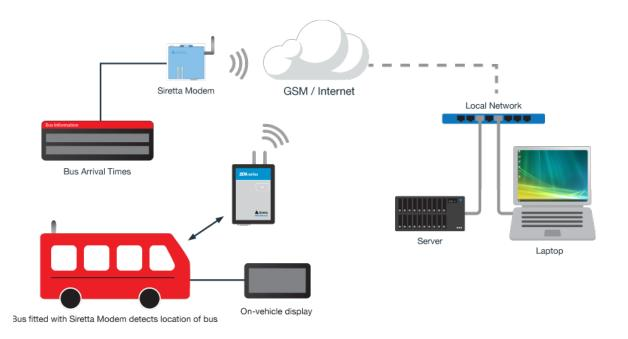
Bus passenger information systems or Real Time Passenger Information (RTPI) systems provide live information about arrival times of buses across a county. The systems use passenger information displays (digital signs) fitted at bus stops and each bus is fitted with a GPS tracking device.
