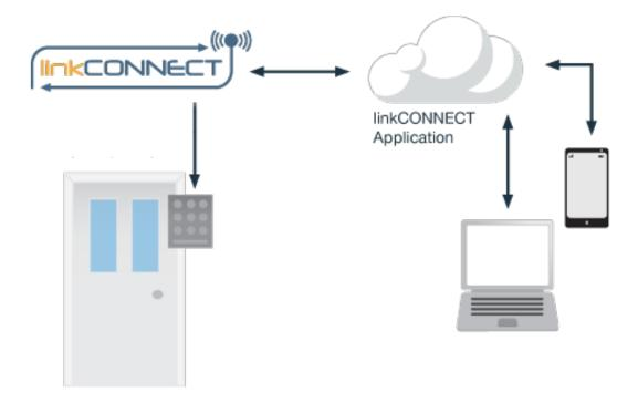
Siretta linkCONNECT solutions are used in remote door entry applications to authenticate users via either a simple pin code entry mechanism or a more advanced system such as fingerprint recognition or Bluetooth phone authentication. Once user is authenticated the system is able to securely grant access to building premises, warehouses, garages etc without the need for a manual key exchange or a lock and key entry.
