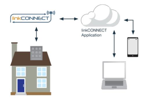
Siretta linkCONNECT solutions are used in home automation projects to link the home to the home owner via a mobile application on their smart phone. The solution uses a remote link to capture information about the status of the home including monitoring lights, doors and windows and total energy usage,
