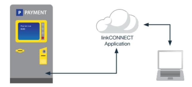
Siretta linkCONNECT solutions are used in automatic payment machines where authorisation to purchase a service is required via credit card payment or validated company credit account. The linkCONNECT solution provides a point to point link to the distribution point and provides a real time device status which can be used to authorise payments and initiate delivery of parking ticket/car park access/congestion charge etc.
