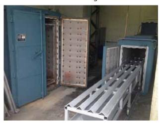
PPSL utilises two bespoke rate controlled ovens to effect the removal of a wide range of contaminants; from everyday paints and coatings, to modern chemical resistant polymers. The first oven in PPSL is a box oven able to accommodate parts up to 1.2 cubic metres. The second oven in PPSL is a screw cleaning oven able to accommodate parts up to 4m in length.
