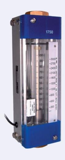
The Series 1750 range of Variable Area Flowmeters are ideal for providing instantaneous flow rate measurement for most process gases and liquids. The standard models are suitable for flows up to 50 lit/min on liquids and 1750 lit/min on gases @ STP.
