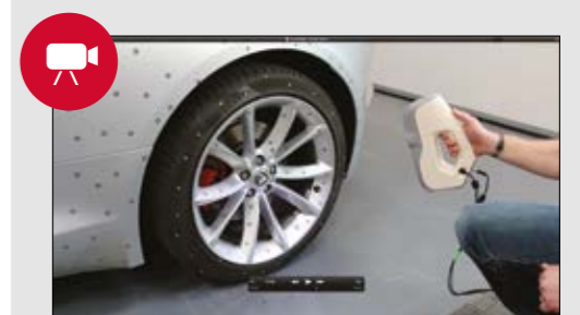
The Eva is also used in conjunction with the Europac3D photogrammetry kit, ScanAlign – a package used to flawlessly scan large industrial components which contain very little geometry over large surface areas. Type europac3d into YouTube to see the ScanAlign video or see the ScanAlign specification on Page 6 .
