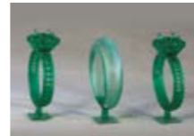
The 1200 is a small object 3D printer using a castable VisiJet Green FTX material
