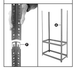
Add remaining side beams and front & back beams to uprights to create the rest of the shelves at the preferred heights
