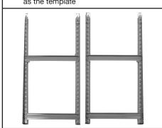
Join the two side frames together using the longer front & back beams
