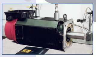
High Speed Balancing to 20,000 RPM+
