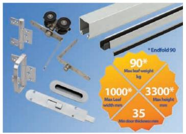
Endfold 50/90 Folding door system suitable for both residential and commercial applications. Features include nylon wheels with bearings, anodised aluminium track, track & floor mounted pivots and a range of hinges and flush bolts either in a satin stainless or polished gold PVD finish. The 90kg replaces pivots with hinges for greater performance.
