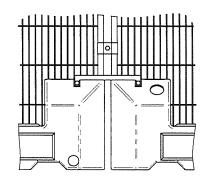
Multiple bays are connected using the supplied braces along with standard panel clamps.
