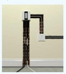
Note - if installing in a bathroom or other 'wet' room the thermostat must be located OUTSIDE of the room on the opposite side of the wall, for example in a bedroom or hallway/landing.
