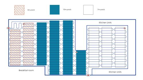
After deciding the route that your power supply cables will take from the mat to the point of supply, cut a 6 mm wide channel in the insulation along this route and drop the power supply cables into this channel. Similarly you have to cut a small section / channel in insulation or laminate depending on the position of Thermostat sensors.
