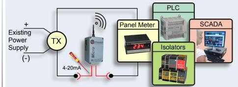
Incorporate the Micro RTU into existing circuits at site, such as digital panel meters, PLCs, Trips Amps, Isolators or local SCADA systems.
