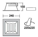
Square recessed luminaires made from aluminium frame - anodised
