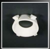
The light housing CERAM 3S is suitable for installation in plasterboard ceilings of 12mm thickness. It is made of cast ceramic material with an inner downlight component of cast aluminium. Versions are offered for 12V halogen, 230V halogen or LED and compact metal halide lamps.
