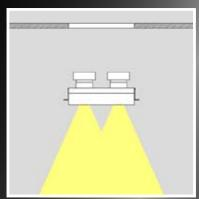
The luminaire ORBIS 2F is suitable for plasterboard ceilings and fits flush for a trimless appearance. It is made of cast aluminium and has a holder system of two steel strings. Two inner bodies may be selected from fixed, adjustable, pinhole and adjustable pinhole options. Versions are available for 230V and 12V halogen and LED lamps.
