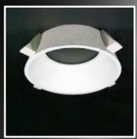
The light housing CERAM 3 is suitable for installation in plasterboard ceilings of 12mm thickness. It is made of cast ceramic material with an inner downlight component of cast aluminium. Versions are offered for 12V halogen, 230V halogen or LED and compact metal halide lamps.
