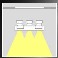
The luminaire ORBIS 3F is suitable for plasterboard ceilings and fits flush for a trimless appearance. It is made of cast aluminium and has a holder system of two steel strings. Two inner bodies may be selected from fixed, adjustable, pinhole and adjustable pinhole options. Versions are available for 230V and 12V halogen and LED lamps.
