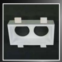
The light housing CERAM 4S2F is suitable for installation in plasterboard ceilings of 12mm thickness. It is made of cast ceramic material with an inner downlight component of cast aluminium. Versions are offered for 12V halogen, 230V halogen or LED and compact metal halide lamps.
