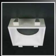
The light housing CERAM 4L is suitable for installation in plasterboard ceilings of 12mm thickness. It is made of cast ceramic material with an inner downlight component of cast aluminium. Versions are offered for 12V halogen, 230V halogen or LED and compact metal halide lamps.
