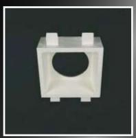
The light housing CERAM 4S is suitable for installation in plasterboard ceilings of 12mm thickness. It is made of cast ceramic material with an inner downlight component of cast aluminium. Versions are offered for 12V halogen, 230V halogen or LED and compact metal halide lamps.
