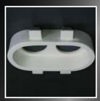
The light housing CERAM 3S2F is suitable for installation in plasterboard ceilings of 12mm thickness. It is made of cast ceramic material with an inner downlight component of cast aluminium. Versions are offered for 12V halogen, 230V halogen or LED and compact metal halide lamps.
