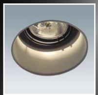
The luminaire JAZZ MAX is suitable for plasterboard ceilings. It is made of cast aluminium. The inner part rotates and tilts. It operates at 230V/50-60Hz. Versions are available for 230V and 12V halogen and LED lamps.
