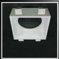
The light housing CERAM 4M is suitable for installation in plasterboard ceilings of 12mm thickness. It is made of cast ceramic material with an inner downlight component of cast aluminium. Versions are offered for 12V halogen, 230V halogen or LED and compact metal halide lamps.
