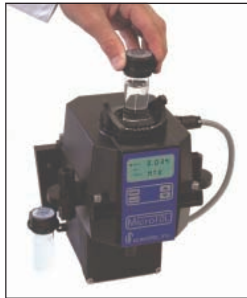
MicroTOL with Calibration Cuvettes A complete primary calibration can be completed in less than five minutes
