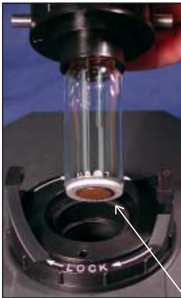
Ultrasonic Cleaning System Keeps the optical chamber clean in finished or raw water applications.
