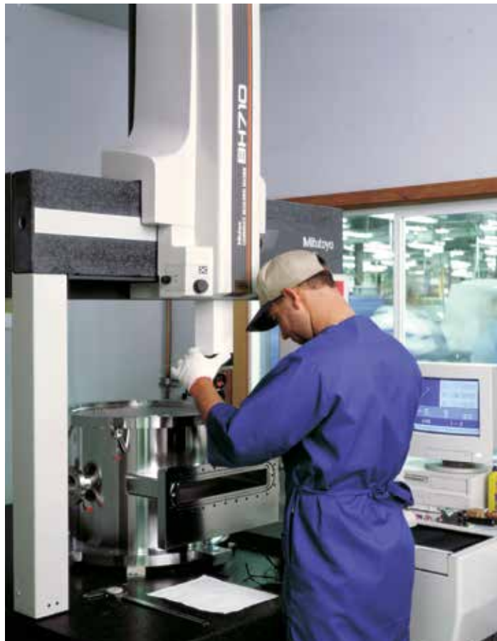
Mechanical inspection of process chamber with CMM
