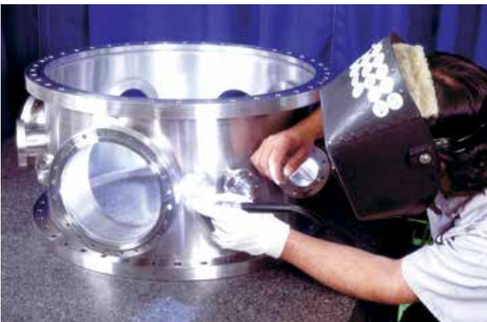
GTAW fusion welding
