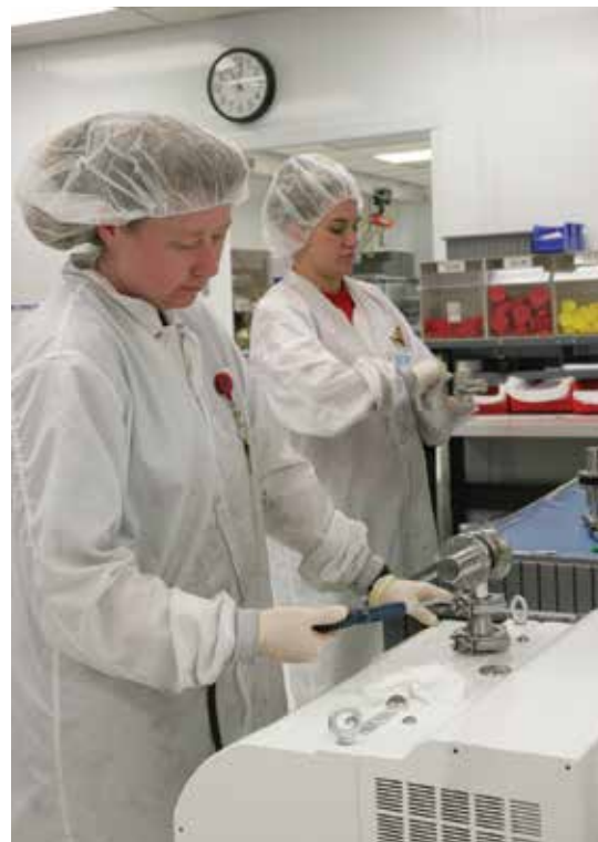
Dry leak detector for valve inspection
