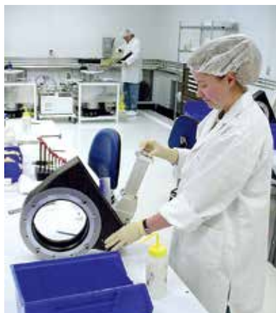
Valve assembly in Class 1000 Clean Room
