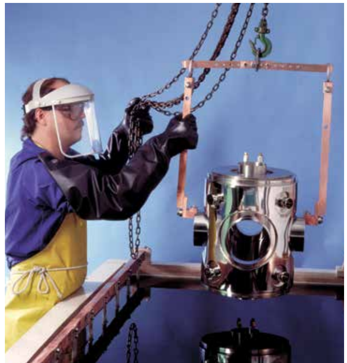
Electropolishing vacuum chamber
