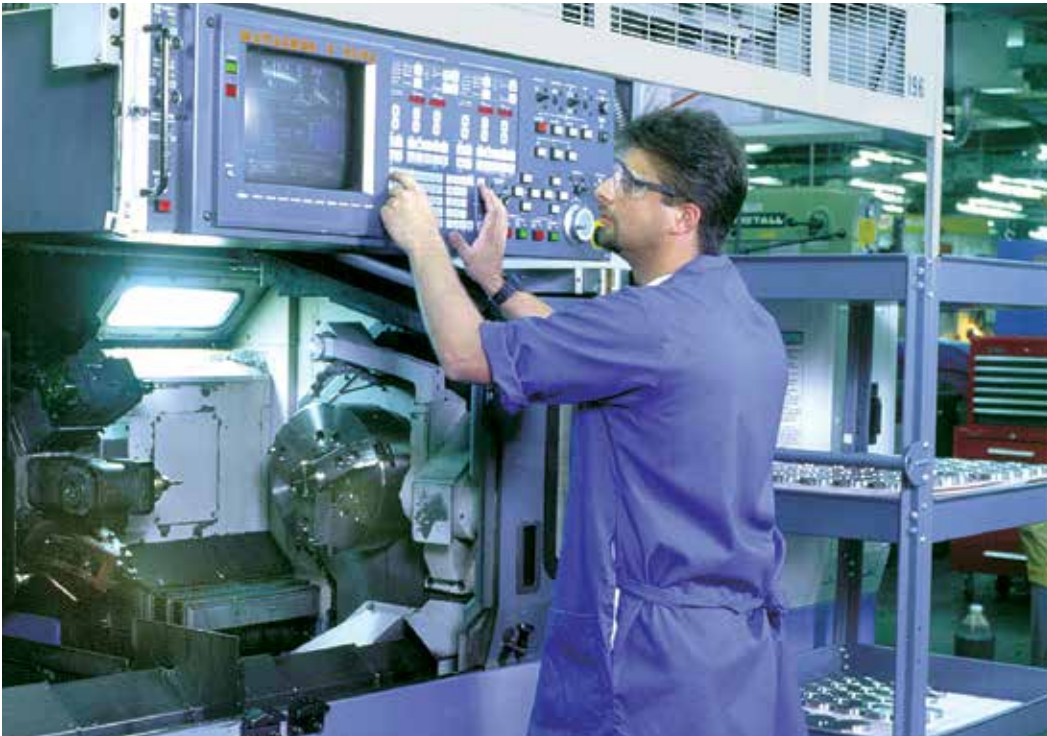
CNC Machining Center with dual spindles, live tooling and robotic gantry
