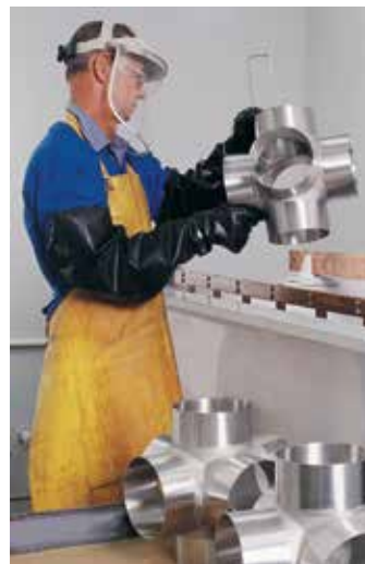
Electropolishing weld fittings
