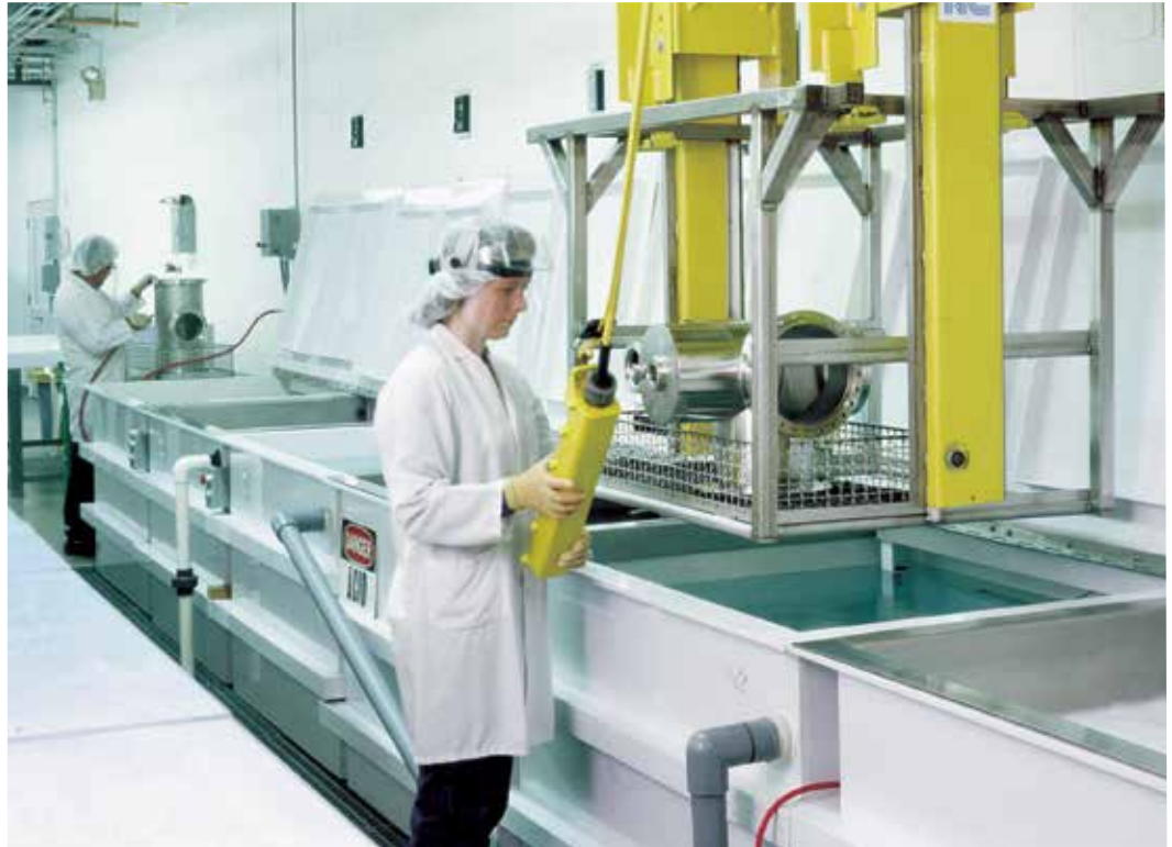
Chem cleaning vacuum chambers
