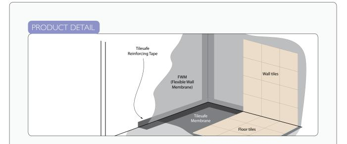
**RIW** FWM - Flexible Wall Membrane is a flexible coating for waterproofing wall surfaces prior to the application of ceramic tiles and natural stone in wetroom and other critical areas.
