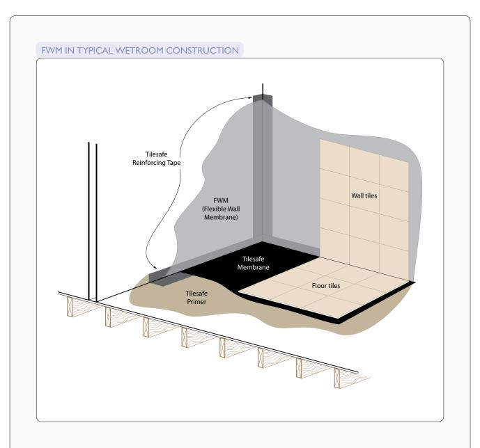
For timber floors we recommend that the Tilesafe membrane is applied to the entire wetroom floor.
