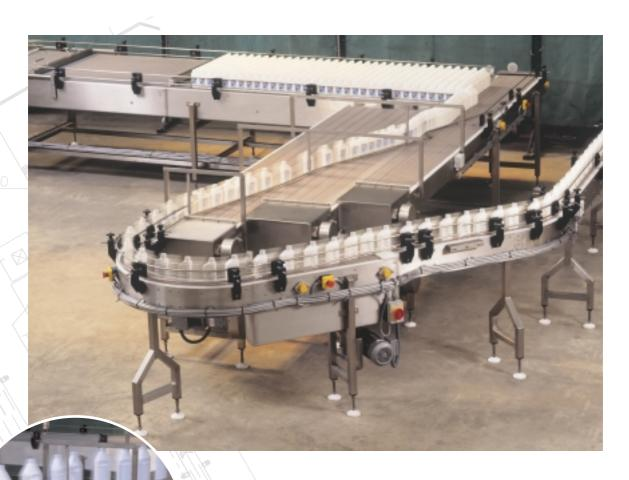
Manufactured from Brushed finish stainless steel or mild steel, our pressureless combiner systems are principally designed to allow a range of pre manufactured products to be manually or automatically unloaded into a system where single file is a prerequisite further into the production line.
