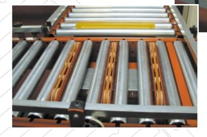
A full range of powered roller conveyors are available, from single units to fully integrated systems. Packages as small as 250mm long can be handled on the modular system with its 37mm diameter close pitch rollers or the more traditional lineshaft type is available with 50mm diameter rollers.
