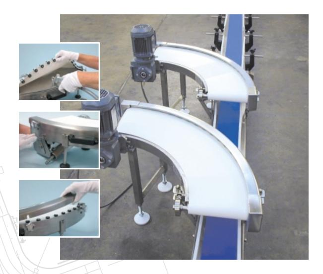
Arnott's belt bend conveyors can be supplied with standard conical end rollers or 15mm diameter knife edges.
