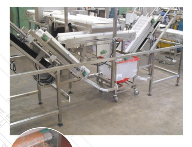
The client's requirement was to transport boiled sweets from the cooling lines to the storage units via a vibratory grading hopper and metal detector to portable storage trolleys.
