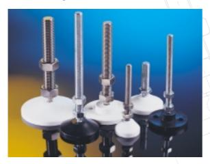
Adjustable feet are available with thread diameter ranging from M10 to M30, the threaded section for which can be supplied zinc plated or stainless steel with thread length to suit individual customer requirements.
