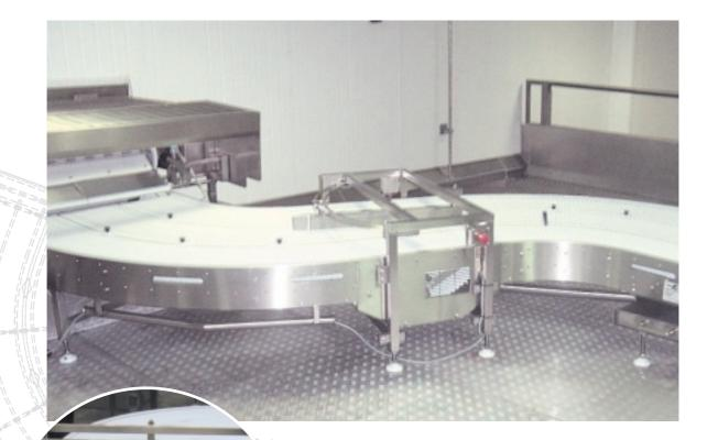
This multilane radius conveyor has replaced two 90° wire belt conveyor bends, plus the connecting conveyor between them.
