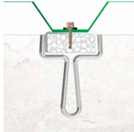
Cross section of a JTB-AR channel profile with self tapping screw holding a sheet metal roof
