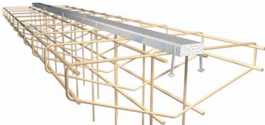
JTB-UNI channel pre-installed in the rebar cage before pouring concrete
