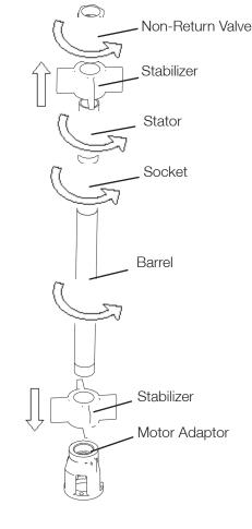
WARNING: When removing the Stator it is very important that the tube is not distorted by pipe wrenches, vice jaws etc. Damage to the outside of the stator tube can result in loss of performance and seizure of the pump.
