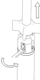
Pull the pump off the rotating assembly being careful to pull in a straight line to prevent damage to the flexishaft coating.
