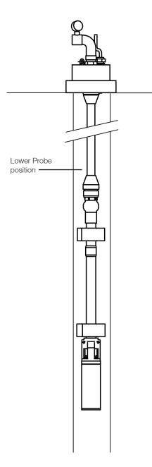
As an initial setting the top probe should be positioned about 1 metre above the bottom probe. It is not necessary to separate the probes by a large distance as it is with some AC pumping systems. (In AC systems the probe separation is used to control the number of pump starts per hour because more than 20 starts per hour can cause the motor to overheat). The Sun-sub system will not be damaged by repeated starts so large separations are not required.
