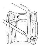
The pump can be installed on various rising main materials including polyethylene pipe. If using a polyethylene rising main Mono Pumps recommend that Class 12 pipe be used with cone type compression couplings. Screw the fitting that connects the pump to the rising main into the threaded outlet on the top of the pump.
