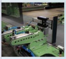
Pack turners fitted with shock-absorbers, integrated with alignment guides; these are customised to suit the particular type and weight of the pack to be handled.
