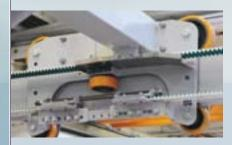
The use of transmission chains and belts has been reduced to maximize reliability. Maintenance-free toothed belts. Minimum noise level and improved accessibility.
