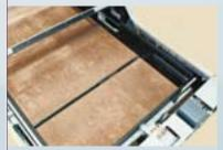
Stripper table split in two halves to reduce strokes. Three independent centering guides for precise, compact layer positioning. Ranprex® low friction and low wear surface coating
