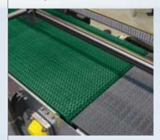
**Double infeed belt** achieved using two modular conveyors with independent motors. Inverter-controlled speed.
