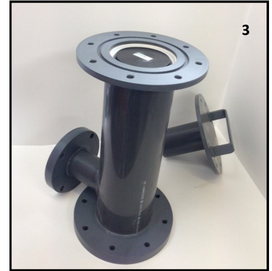
HEPA Filter (clean) now in the unit, unit requires 2 HEPA filters in order to be in the correct place. 1 working and 1 on standby.
