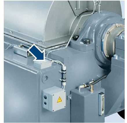
Vibration monitoring (standard)
