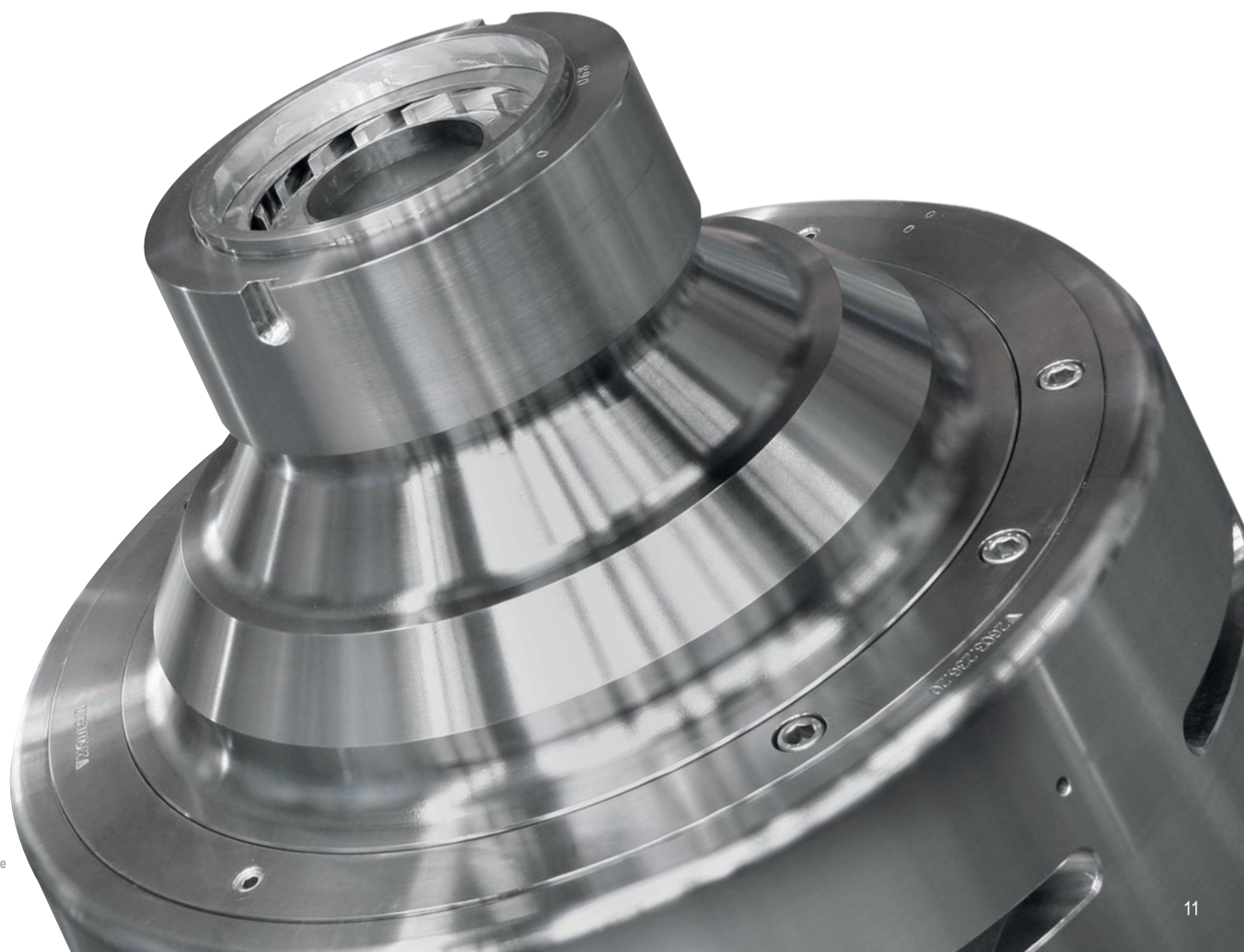
The picture shows the bowl of a disc stack centrifuge
