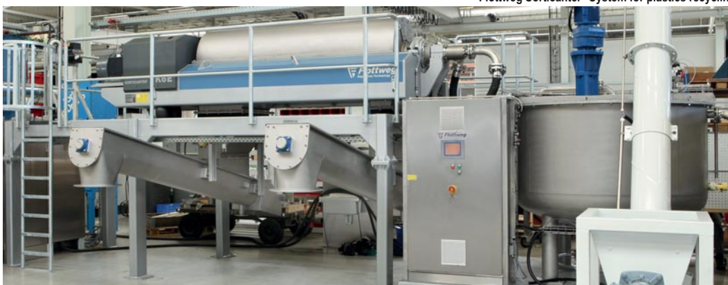
Flottweg Sorticanter® System for plastics recycling
