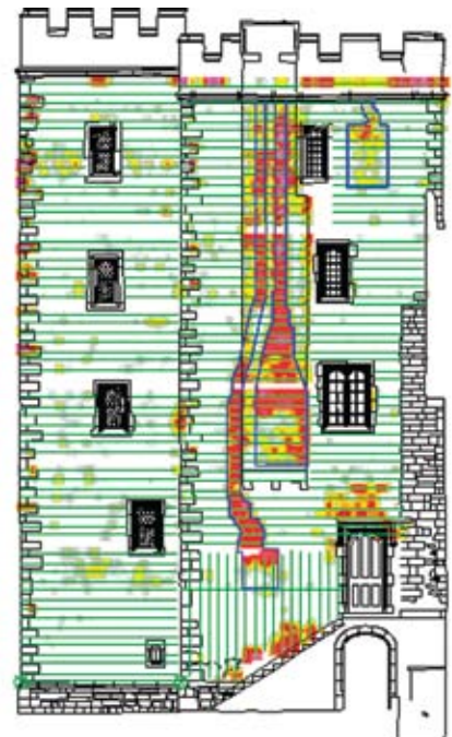
Mapping voids in masonry walls, UK
