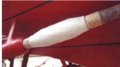
A typical ropeguard and coupling cover after docking, shown here on HMS Westminster (Courtesy UK MoD)
