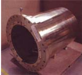
Both the intermediate (pictured above) and aft bearings were fitted with thermocouples to monitor the bearing surface temperature during the basin trials
