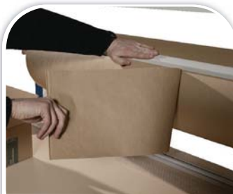
Tear bar allows paper to be easily torn to size
