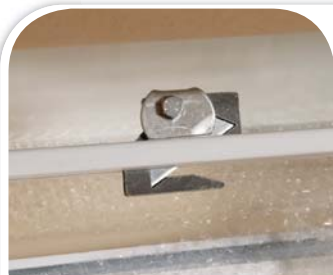
Cutting bar has integral blade attachment
