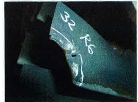
Fig. 6. Compressor blade damage resulting from initial component failure.
