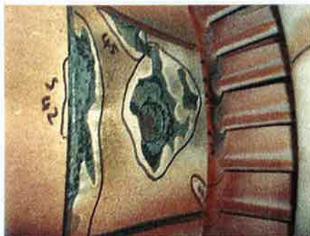
Fig. 3. Thermal barrier coating spallation and base material oxidation.
