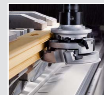
Full power: Main spindle with up to 30 kW
