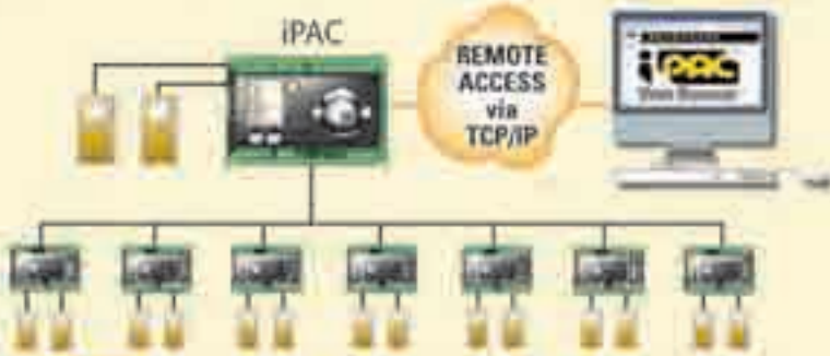
Up to 16 doors when you combine the iPAC with up to 7 PAC 512 controllers
