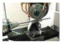
· P-axis with CNC force controlled tailstock
