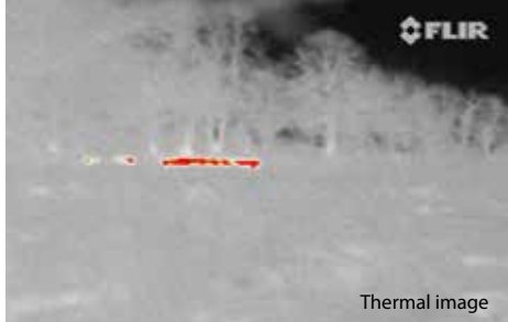
These deer are easy to spot thanks to the InstAlert™ feature, which colors the hottest part in the thermal image red, available on all FLIR Scout PS-Series.
