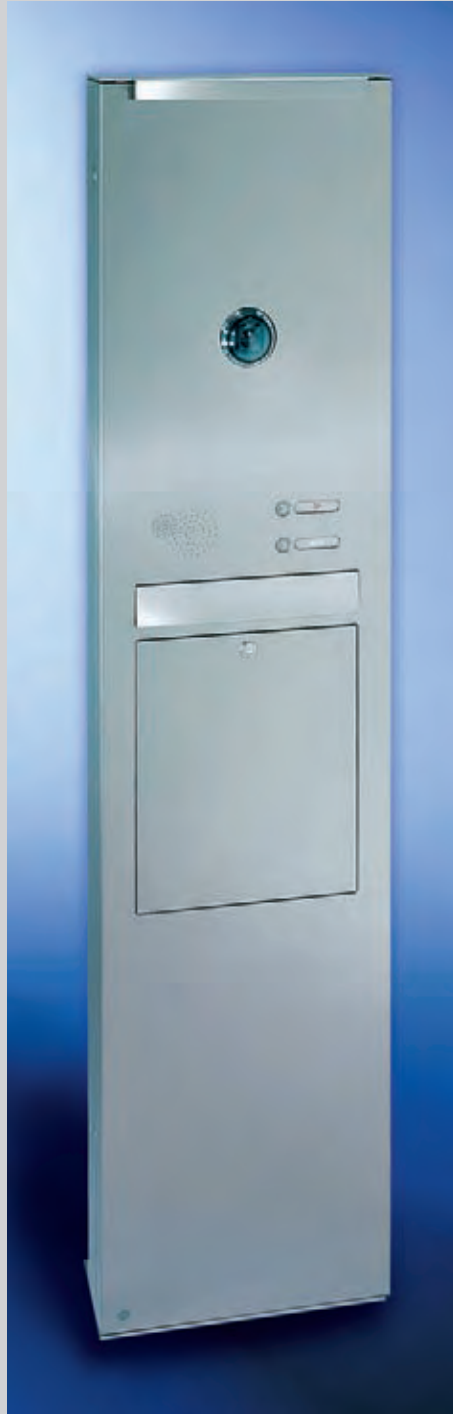
Commercial Line. V4A stainless steel pillar shaped mail box, one-part mail box unit with RSA , inclined opening 335 x 50 mm, box size 335 x 770 x 140 mm, front mail removal door 335 x 440 mm bottom hung with two opening restrictors, fitted with LED lighting and CCTV camera supplied by others, pillar height 2000 mm.
